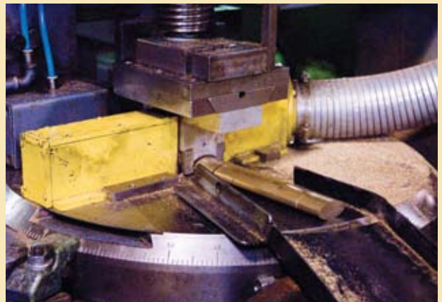
▲ One of the first production steps is cutting the lock body to length from an extruded brass bar. This saw was built in-house specifically for this operation.
